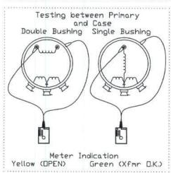
The diagrams below, for single and double bushing capacitors, show various connections when using the 6793 tester. We have shown the reading that will be obtained 'IF' the capacitor is good.
